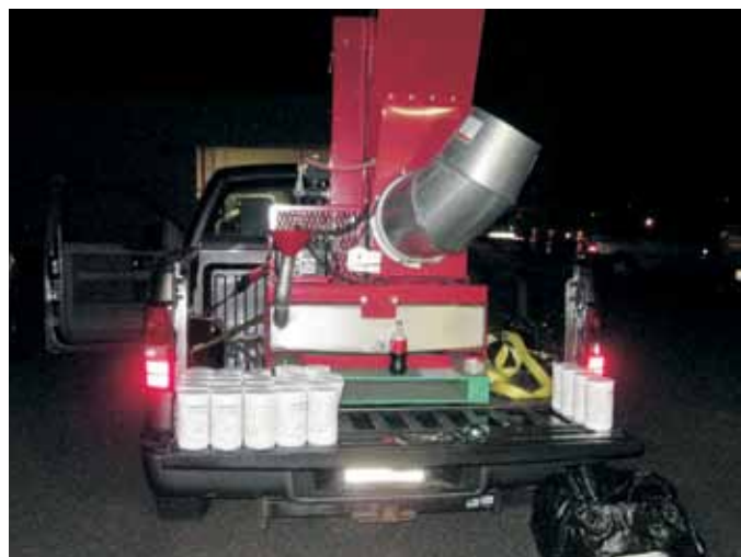
Monmouth and Mercer mosquito control staff experimented with truck-mounted sprayers to deliver larvicides, such as VectoBac® WDG, to container habitats in large treatment sites that are difficult to access.
