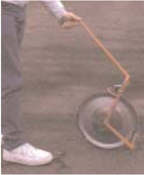
Swath width is best determined by doing a static test on a flat, relatively clean surface such as a parking lot.
