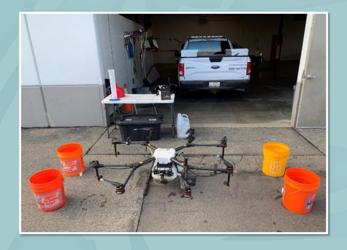
DJI AGRAS MG-1s controller has a flow calibration function.
