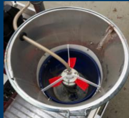
Calibrated the turbine at full speed (WOT) to deliver 3.2 gallons per minute @ 50 PSI
