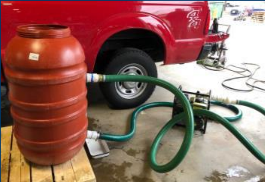
Mixed 1 pound Vectolex WDG per gallon of water for a 12% W:V solution
